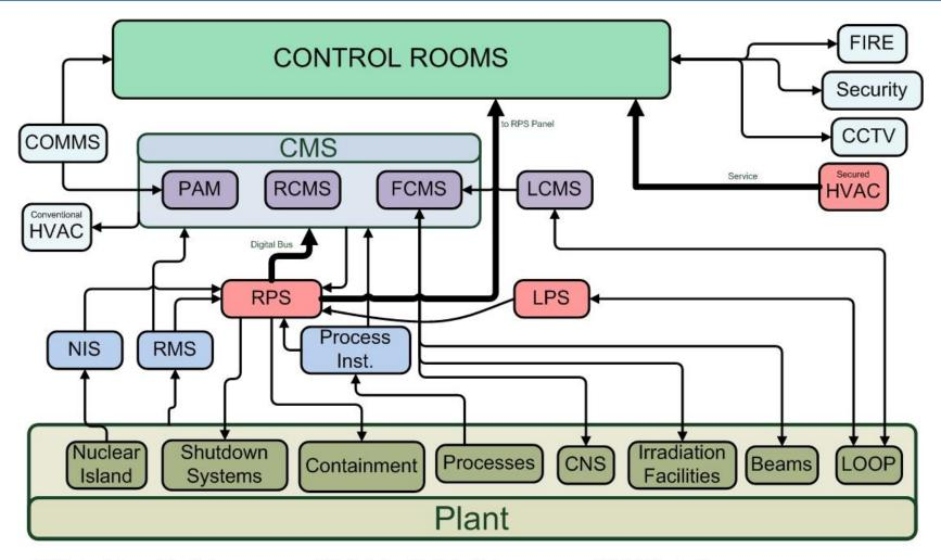
NIS: Nuclear Instrumentation System RMS: Radiation Monitoring System RPS: Reactor Protection System PAM: Post Accident Monitoring RCMS: Reactor Control and Monitoring System FCMS: Facilities Control and Monitoring System
